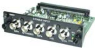
Image 1-1 5 Cable input (Multi purpose) (R9854430).
